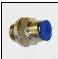
Part no. 14878 1/8" BSP Mark Stud straight fitting to 4mm air pipe.
